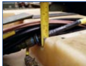
Photograph 1 shows Insufficient space to accommodate Bowman cabling, due to a smaller than expected recess in the fuel tank of a Warrior armoured vehicle. This is difficult
