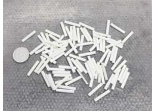
A number of Beta-lights (luminescent objects used as light sources), and a five pence piece to show the scale. Beta-lights are manufactured in several shapes and sizes.
