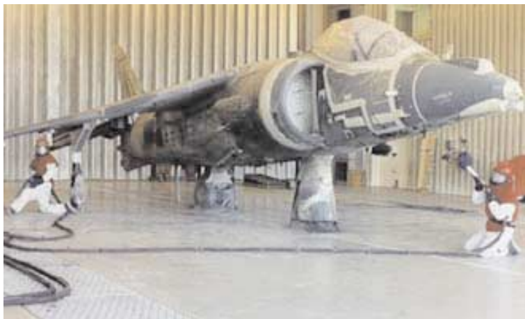
A Harrier being stripped using plastic media. All openings and areas susceptible to damage are covered to prevent the plastic media penetrating the fuselage and damaging the aircraft.
