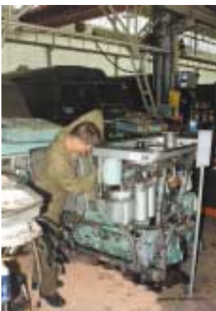
REME Engineer repairing a powerpack
