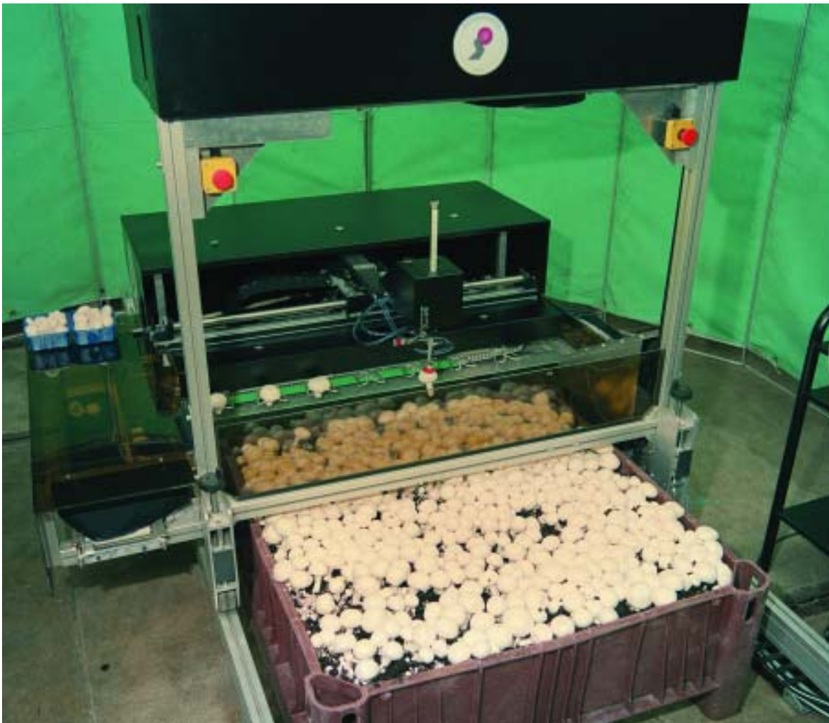
Robotic Mushroom Harvester. Photograph courtesy of Silsoe Research Institute.
