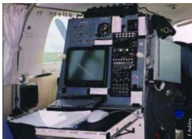
Data recording station within an aerial surveillance aircraft
